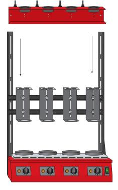
► Fasten the condenser stand in place with the pair of knurled screws provided.
