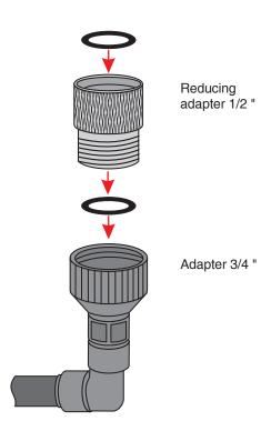
The connection for the cooling water outflow (3, figure on previous page) is likewise located on the rear of the cooling water distributor with condenser stand.
