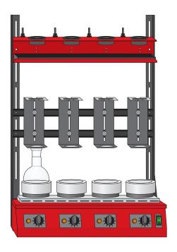
Insert the extractors from above into the extractor mounts and seat them on the round bottom flasks.
