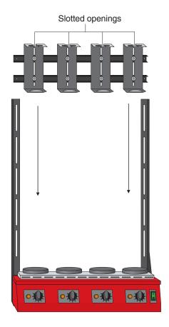
► Fasten the horizontal support bars with the four knurled screws provided.
