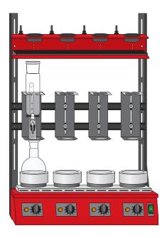
Insert the reflux condensers onto the extractors.
