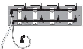
The connection for the cooling water supply hose is found on the rear of the condenser stand.
